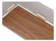
3. The end joints of the planks in the first row are assembled by inserting the tongue side into the groove side of the previous plank at a natural angle. Gradually lower the plank down flat until the end joint closes with no gap, insuring that the planks are perfectly aligned at the top and bottom of the joint. Install remaining full planks in the first row.
